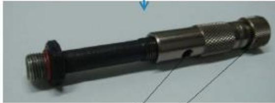
Air leaks through these holes      Turn the knob to withdraw the core valve
